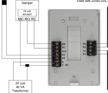
R - 24vac power input C - 2vac power common RO - damper run open signal RC - damper run closed signal MC - 24V motor common DS - duct temperature sensor DS - duct temperature sensor
