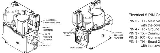
Electrical 5 PIN Connector Pin Out
