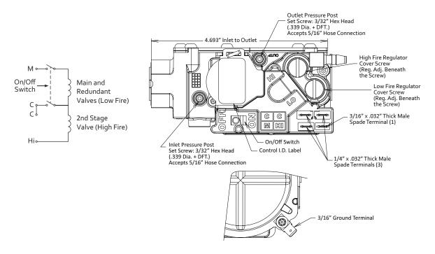
Fig. 2 - Two-Stage Valve Features, Terminals and Wiring
