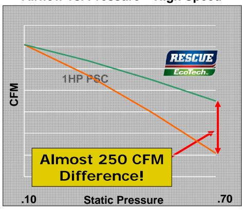
Works To Maintain Airflow As Static Pressure Increases From:
