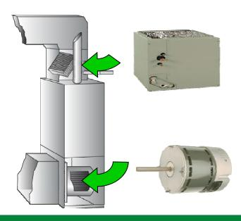
Upgrade Blower When Replacing A/C
