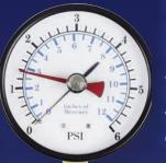
Use to pressure test all new installations for UNIWELD EMPLOYS leaks and inspection codes. After installation and the system has been pressurized, the leakage will be indicated by a pressure drop on the gauge.
