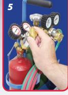
STEP 51 To shut down the torch for storage or transportation, close the torch valve [vent safely]. valves tightly and secure
