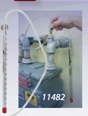
Uniweld Gas Pressure Test Kits include: A Diaphragm Gauge that accurately sets manifold pressure for Natural or LP gas; a Brass Fitting (barbed x 1/8" M.P.T.) and rubber tube with nipple for easy connection; Molded Plastic Case; Instructions.
