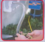
3. Allow Nitrogen to flow through **Sludge Sucker®** fitting and then watch the sludge get sucked out of the drain line and blown onto the ground.
