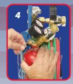
[STEP 4] When you have completed the job and are ready to shut off the torch,always shut the oxygen valve first and then the fuel gas valve [acetylene]. NOTE: Shutting off the fuel gas first can cause backfire first can cause backfire and/or flashback.
