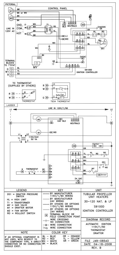
Figure 11C - Tubular Propeller Units 60-120 with Natural and Propane (LP) Gas with Optional Two Stage Gas Control and Honeywell Control Board
