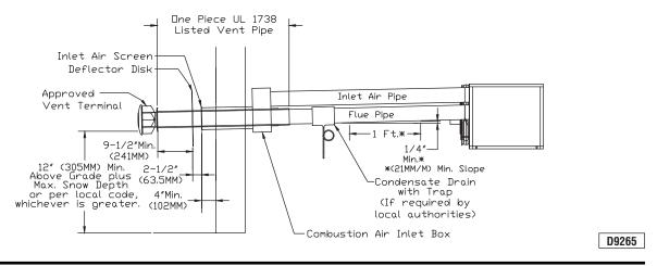
Figure 21 - Horizontal Intake/Vent Installation
