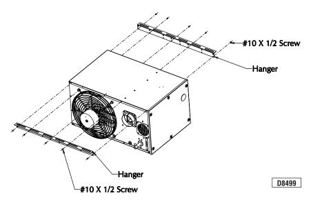
Install Hangers To Front And Rear Of Unit With #10 X 1/2 Screws (10) Plcs As Shown
