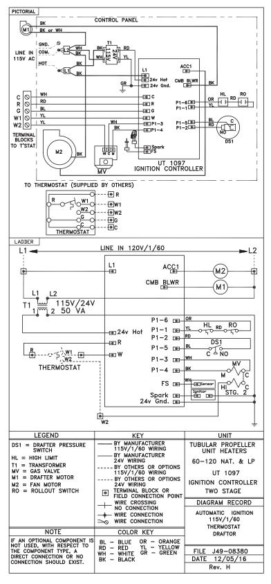
Figure 11B - Tubular Propeller Units 30-120 with Natural and Propane (LP) Gas with Single Stage Gas Control and Honeywell Control Board
