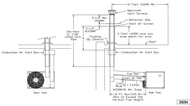
Figure 20 - Horizontal Intake/Vent Installation
