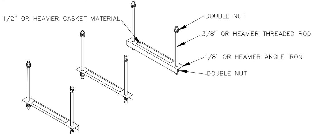
**Figure 1: Recommended Support Frame for Horizontal / Counterflow Furnaces**
