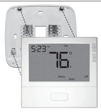
Align the 4 tabs on the subbase with corresponding slots on the back of the thermostat, then push gently until the thermostat snaps in place.
