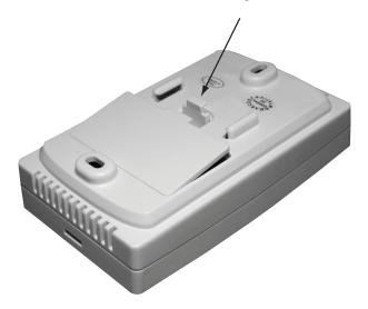
Once you have removed the door from the back of the remote, insert 2 AA Alkaline batteries and replace the battery door.
