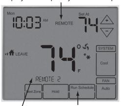
The name of the remote sensor will be displayed. In this example, it is **REMOTE 2**.
