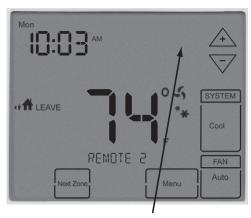
Setpoint will only be displayed for the zone currently being used by the program or in hold. Press the  $\triangle$  or  $\nabla$  to show the setpoint for adjustment.
