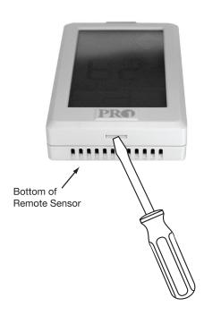
Once you have removed the RZ251W from the subbase, insert 2 AA Alkaline batteries.
