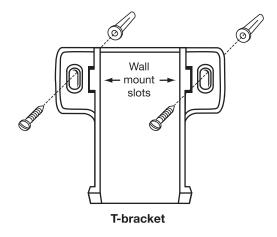
Slide the Remote Sensor over the mounted T-bracket.
