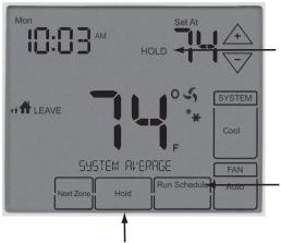
To put the thermostat into hold select system average or the zone you want to hold. Then use the arrows to adjust the setpoint. Then press the **HOLD** key.
