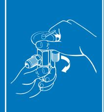
(7) After hand tight, turn element clockwise 60° (or movement equal
