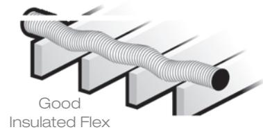
\*A straight run over joists is better than the duct 'dipping' into each joist bay which will increase static pressure and, eventually, deposit water in the 'dips'.
