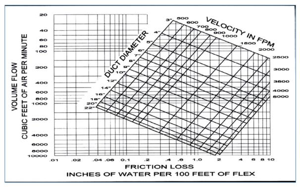
Friction Loss Slide Chart Calculators are available at a minimum cost
