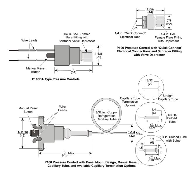
Figure 2: Typical P100 Pressure Control Dimensions, in. (mm)
