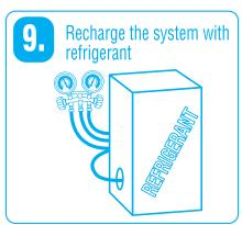
Adjust the refrigerant charge to designed sub cooling if the system is equipped with an expansion valve or compressor superheat if equipped with a fixed orifice or cap tube.
