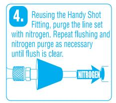
After flushing is completed, purge the tubing with approx.100 psig of nitrogen to push any remaining flush from the tubing
