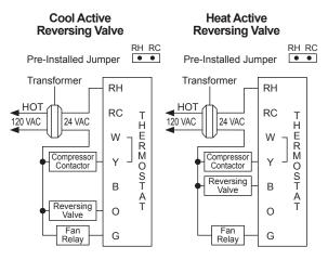
**\*\* Note:** Place jumper between "W" and "Y" terminals. Place heat pump jumper to HP position.
