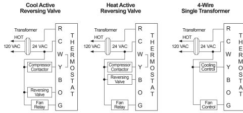
\*\* Note: Place jumper between "W" and "Y" terminals. Place heat pump jumper to HP position. \*\* Note: Millivolt system may require a transformer and/or an isolation relay to operate properly
