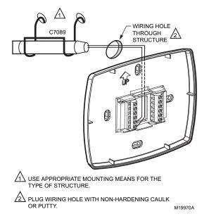
Fig. 26. Wire C7089U Outdoor Sensor to the thermostat.
