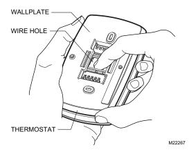
Fig. 7. Separate wallplate from thermostat.
