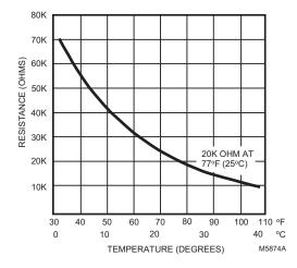
Fig. 44. 20K ohm sensor resistance versus temperature.
