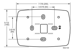
Fig. 2. 32003796-001 Cover Plate dimensions in in. (mm).
