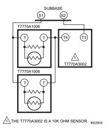
Fig. 29. Wiring two T7770A1006 (20K ohm) Sensors and one T7770A3002 (10K ohm) sensor to provide a temperature averaging network
