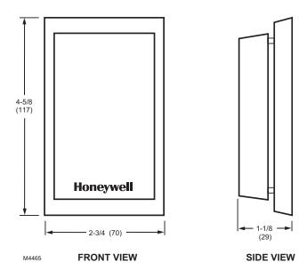
Fig. 5. C7189U Indoor Sensor dimensions in in. (mm).
