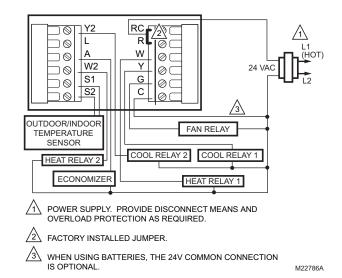
Fig. 17. Typical hookup of single transformer multistage system (up to 2H/2C).
