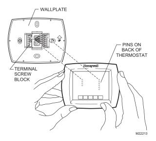
Fig. 41. Placing thermostat back onto subbase.
