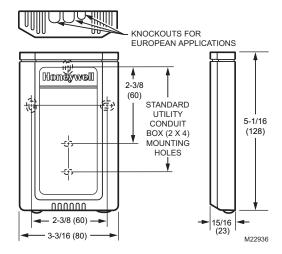
Fig. 4. T7770A dimensions in in. (mm).
