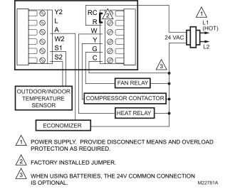
Fig. 12. Typical wiring of single transformer 1H/1C system.
