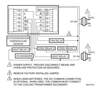
Fig. 18. Typical hookup of dual transformer multistage system (up to 2H/2C).
