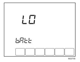
Fig. 39. Low battery signal.
