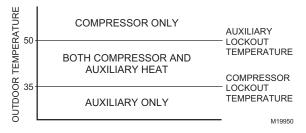
Fig. 42. Heat Pump Operation with Lockout Temperatures
