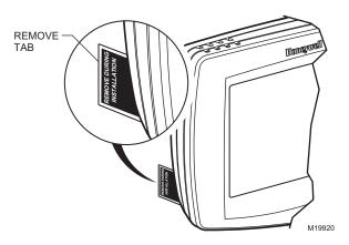
Fig. 24. Remove tab labeled REMOVE from thermostat back.
