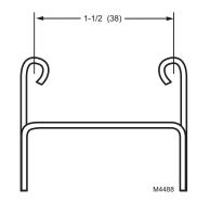
Fig. 3. C7089U Outdoor Sensor Mounting Clip dimensions in in. (mm).
