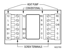
Fig. 9. Terminal identifications for system type.
