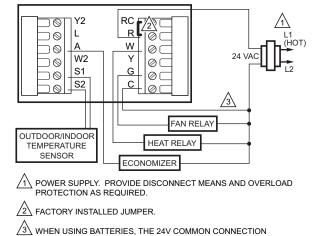
Fig. 15. Typical hookup of heat-only system with fan.
