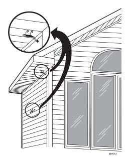
Fig. 25. Typical locations for C7089U Outdoor Sensor.
