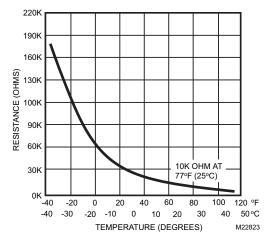
Fig. 43. 10K ohm sensor resistance versus temperature.
