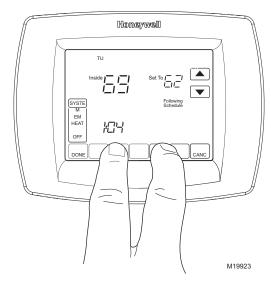
Fig. 32. Entering Installer Setup.
