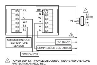
WHEN USING BATTERIES, THE 24V COMMON CONNECTION IS OPTIONAL.
