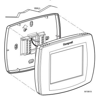
Fig. 40. Removing thermostat from subbase.
