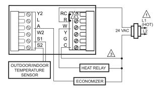
POWER SUPPLY. PROVIDE DISCONNECT MEANS AND OVERLOAD PROTECTION AS REQUIRED.
