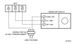
Fig. 5. Wiring SPC to control CDO-51 or MARD damper in bypass application.
