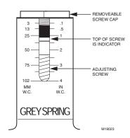
Fig. 6. Static pressure range settings.
