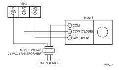
Fig. 4. Wiring SPC to control ML6161 Actuator in a bypass application.
