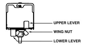
Fig. 4. Air Flow Adjustment
