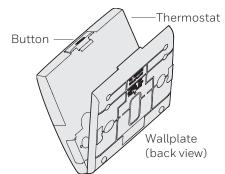
2 Mount wallplate as shown. Mount new wallplate using screws and anchors included with the thermostat. Drill 3/16-in holes for drywall.
