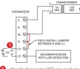
Wire the thermostat IAQ relay to the low speed fan for dehumidification control at the equipment. The thermostat relay can be set to normally open or normally closed in the thermostat installer setup.
