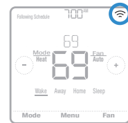
Example of Wi-Fi is connected.
