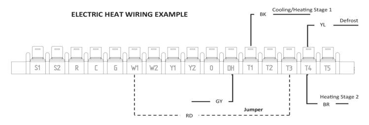
\*Move BROWN (BR) wire from TB1-T2 to T3, T4 or T5 to change blower speed during heating stage 2 operation. YELLOW wire from blower relay BR1 to TB1-T2 must be moved to the same position as the BROWN (BR) wire.
