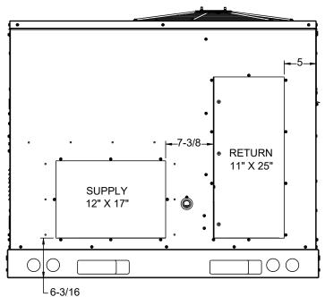
HORIZONTAL DISCHARGE DUCT CONNECTIONS
