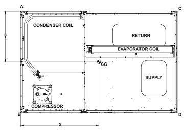
CORNER AND CENTER OF GRAVITY LOCATIONS NOTE: UNIT SHOULD BE LIFTED AT A POINT ABOVE CENTER OF GRAVITY.
