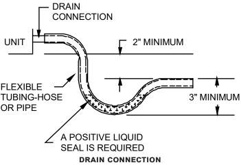
Install condensate drain trap as shown. Use 3/4" drain line and fittings or larger. Do not operate without trap.
