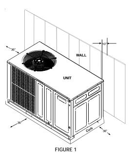
The unit should be set on a solid, level foundation - preferably a concrete slab at least 4 inches thick. The slab should be above ground level and surrounded by a graveled area for good drainage. Any slab used as a unit's foundation should not adjoin the building as it is possible that sound and vibration may be transmitted to the structure. For rooftop installation, steel or treated wood beams should be used as unit support for load distribution.
