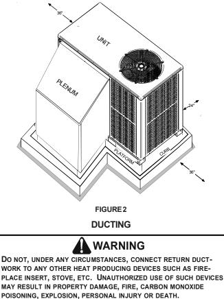
Ducting work should be fabricated by the installing contractor in accordance with local codes. Industry manuals may be used as a guide when sizing and designing the duct systemsuch as NESCA (National Environmental Systems Contractors Association, 1501 Wilson Blvd., Arlington, Virginia 22209).
