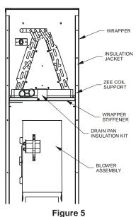
**NOTE:** When converted to downflow position the coil may protrude above the cabinet on some models.
