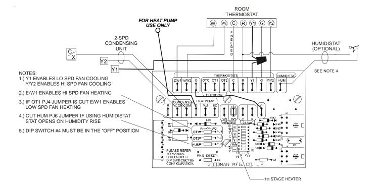
2 SPD COOLING ONLY - WITH 2 STAGE HEAT THERMOSTAT
