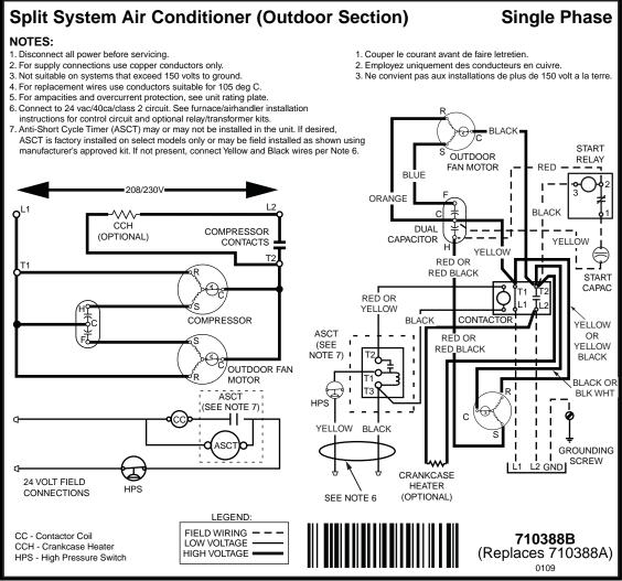
Figure 4. Wiring Diagram for 1.5 - 4 Ton Models (without CoreSense<sup>™</sup>)
