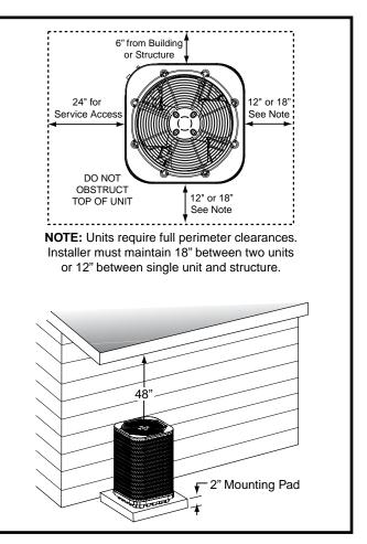
Figure 1. Clearance Requirements
