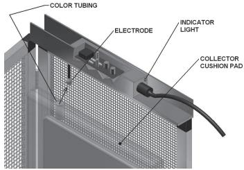
Fig. 3 Collector Pad Replacement
