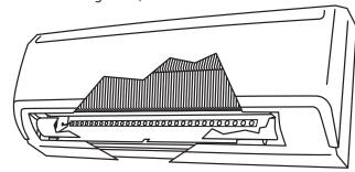
Cutaway view of typical Mini UV LED® installation in mini split
