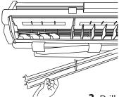
**2b.** For systems with non-removable drain pan, remove louvers and baffles to access the area behind.
