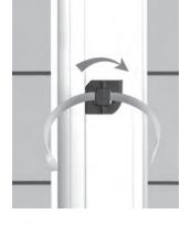
(3) Position and twist in lineset duct clips (Model# LDC) evenly spaced throughout installation. Nylon cable ties (not included) slip through lineset duct clips and fasten around lineset.
