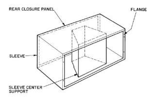
Fig. 1 - Wall Sleeve with Center Support and Rear Closure Panel
