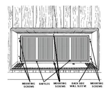
Fig. 4 - Securing Grille to Wall Sleeve
