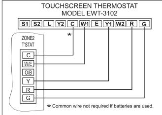
*Figure 2b.* Model EWC-3102: Configured for 1 heat 1 cool (SS1 mode). Can be configured for heat pump. See thermostat instructions for further details.
