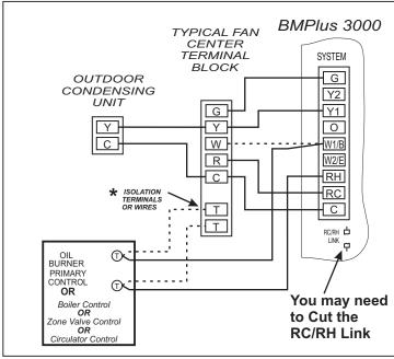
Figure 8 Two transformer Oil or Hydronic / A/C system.
