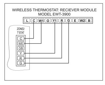
*Figure 3* Model EWT-3900: Wireless Thermostat. Configured for 1 heat 1 cool (SS1 mode). Can be configured for heat pump. See thermostat instructions for further details.
