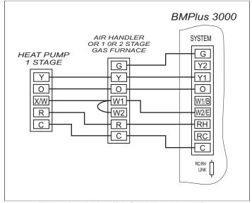
Figure 9 -- 2 Heat / 1 Cool Heat Pump System
