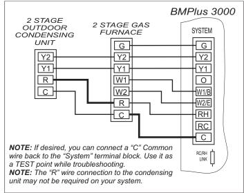
Figure 11 Single transformer 2 Stage Heat & Cool system
