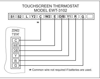
*Figure 2d.* Model EWC-3102: configured for 2 heat 1 cool heat pump (HP1 mode). See thermostat instructions for further details.
