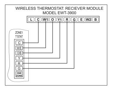
*Figure 4* Model EWT-3900: Wireless Thermostat. Configured for 2 heat 1 cool heat pump (HP1 mode.)See thermostat instructions for further details.
