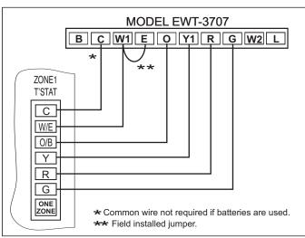
*Figure 2c.* Model EWT-3707: Configured for 2 heat 1 cool heat pump (HP1 mode). See thermostat for further details.
