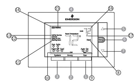
Whenever "I Replace" appears in the display, new premium brand AA alkaline batteries should be installed. If the house will be unoccupied for an extended period and either "I replace" is displayed, install new batteries before leaving.
