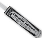
PBACZVOC contains Zero VOC and is ideal for use with PBH Dynastick Hangers. Place a small amount of PBACZVOC on a perforated base and firmly press the hanger against the duct surface. Allow the PBACZVOC mastic to dry, then, impale the insulation over the hanger nail and slip on a locking washer. Duro Dyne PBACZVOC adheres to concrete, metal or wood surfaces and performs in Temperatures Up To 225°F.
