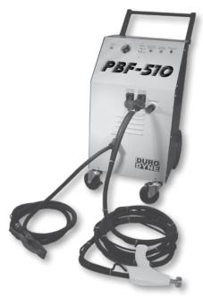
The PBF will weld pins from ½"-2" on 16-28 gauge; weld performance for pins longer than 2" may vary dependent upon voltage, amperage and cable length. It requires 220 volt, 50 to 60 hz service fused for 100 amps. Place a pin on the magnetic tip, insert the pin through the insulation, give the pin a 1/4 twist and depress the trigger switch. For PN type fasteners use a TP2 tip.
