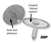
Gold Seal (SSP) pins are considered self sealing pins due to a heat activated gold adhesive on the underside of the washer which secures the pin to the liner facing during the welding process. Gold Seal Pins also feature "dished washers".
