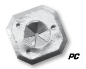
PC Spotter Clips are manufactured of 30 gauge galvanized steel and are used for securing insulation with PN spotter pins.
