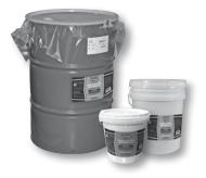
Water-based Insulation Adhesive specifically designed for Spray, Roller and Brush application. WIT is white in color when applied but dries clear for a clean look. WIT features good wet tack, is non-flammable both in the wet and dry state and is classified by UL (file#R5286). Available in 1 gallon pails, 5 gallon pails and 55 gallon drums.
