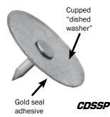
Capacitor Discharge Gold Seal (CDSSP) pins were designed to work perfectly with our Capacitor Discharge Spotwelders. They feature a heat activated gold adhesive on the underside of the washer which secures the pin to the liner facing during the welding process. CDSSP pins are manufactured from 12 gauge steel and feature a "dished washer".
