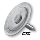
Sloped Washer (CTC) pins are low cost insulation fasteners designed to provide a strong mechanical anchor point for duct liner and a smooth transition from the insulation surface to the quilting depression.
