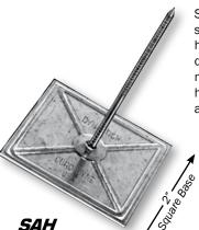
SAH Dynastick is an insulation hanger with a selfstick base. Just peel the release paper from the hanger base and firmly press the base to the clean duct surface. Impale the insulation over the hanger nail and slip on the locking washer. Self-stick
