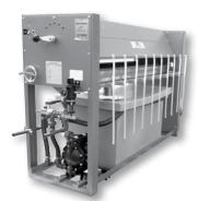
The GBAC applies Duro Dyne WIT or WSA water base adhesive to insulation in preparation for application to sheet metal. It requires 110v service fused for 15 amps. A source of air is required. Please specify the direction of work flow when ordering.
