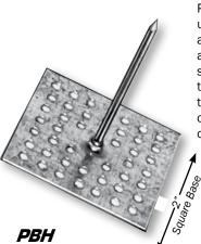
PBH Dynastick is a perforated base hanger for use with super strength PBA mastic. Simply place a small amount of PBA on a perforated base and firmly press the hanger against the duct surface. Allow the PBA mastic to dry, then, impale the insulation over the hanger nail and slip on the locking washer. Duro Dyne PBA adheres to concrete, metal or wood surfaces and withstands constant temperatures up to 180°F.
