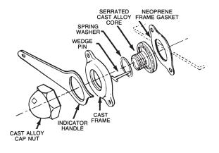
•All SR and SRH type regulators include a cast alloy frame and a neoprene frame gasket.
