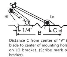
Distance C from center of "V" in blade to center of mounting holes on LO bracket. (Scribe mark on bracket).
