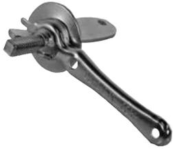
These efficient, low cost, heavy gauge, plated steel regulators install in a "jiffy" by slipping the washer and handle over the threaded square end bearing. The wing nut locks the damper in position. The position of the handle indicates the position of the damper in the duct. For use on round or square ducts.
