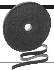
Wherever flanges are used in connecting parts of a duct system, the potential for air leakage exists. Besides contributing to energy waste, leaks can also create noise. Sealing of ductwork can be accomplished with the use of gasket which adheres to flanged surfaces. When this material is attached to a flange, which is then assembled to a second flange, the material is compressed and fills gaps and irregularities creating a seal.
