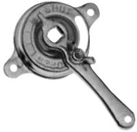
These heavy gauge plated steel regulators are among the most popular on the market. They minimize air leakage and reduce rattle. A wing nut locks the damper in position, yet permits quick readjustment. The dial shows the damper position at a glance. The regulator mounts easily on round or square ducts.
