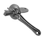
These efficient, low cost, heavy gauge, plated steel regulators install in a "jiffy" by slipping the washer and handle over the threaded square end bearing. The wing nut locks the damper in position. The position of the handle indicates the position of the damper in the duct. For use on round or square ducts.
