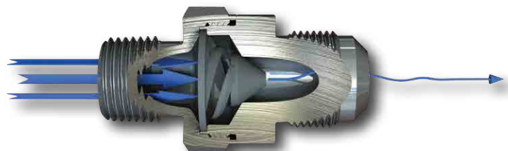
Gas flow is restricted by the plunger due to full line rupture or disconnect providing protection against excessive gas leaks
