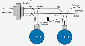
The contacts of the Wet Switch's relay may be wired to use multiple Wet Switches. The drawing above shows the contacts interrupting the 24 VAC signal when either Wet Switch® gets wet.
