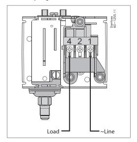
Wire dimensions: 10 AWG max. Cable entry:  $\frac{1}{2}$  in. cable entry for  $\frac{1}{2}$  in. male pipe thread connection (conduit boss) or similar (Pg13.5 or Pg16) screwed
