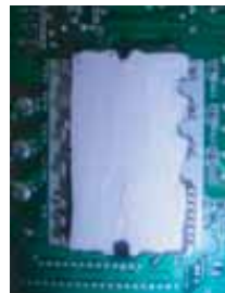
OK : Evenly applied silicon grease.
