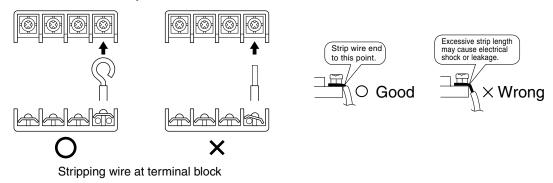
3) Pull the wire and make sure that it does not disconnect. Then fix the wire in place with a wire stop.
