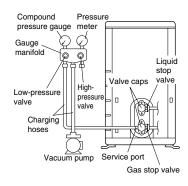
Connect projection side of charging hose (which comes from gauge manifold) to gas stop valve's service port.
