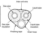
3) Use separate thermal insulation pipes for gas and liquid refrigerant pipes.
