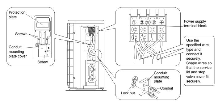
Observe the notes mentioned following when wiring to the power supply terminal board.
