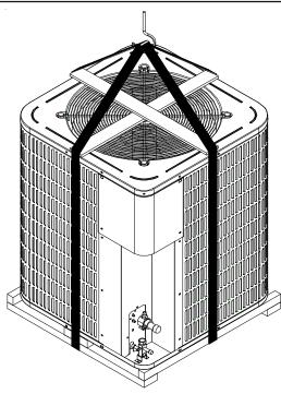
Use field-supplied spreader bars when lifting the unit to minimize the possibility of lifting cable/straps damage. To protect the cabinet louvers, use protective material such as plywood behind the cable/straps. Arrange the straps to form a central suspension point. **NOTE:** When raising and setting the unit, observe all safety rules. Remove shipping skid and all protection and lifting material after the unit is in place.
