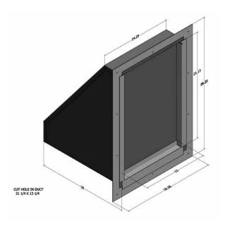
Power Exhaust for 208/230v Units — #DPE901502 Power Exhaust for 460v Units — #DPE901504 Power Exhaust for 575v Units — #DPE901507
