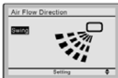
Air Flow Direction (up/down)
