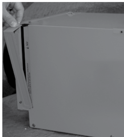
Figure 11: Replace filter door by inserting the bottom tab into the slot, aligning the door and pushing it gently against the unit until the snap button secures the door.
