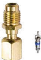
PART# CD8725 PKG QTY: 2 The CD8725 has a gasket in the 1/4" hex nut. The valve body is stationary. When threads of existing system fittings are stripped and anew core won't go in, use this. It has a core and no depressor tip
