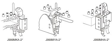
\* Mount pilot ignition port 3/8 in. (9.53 mm) above and 1/4 in. (6.35 mm) away from the center of nearest burner port.
