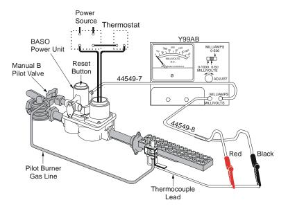
Figure 2: Turn Down Test Using Y99AB Test Kit
