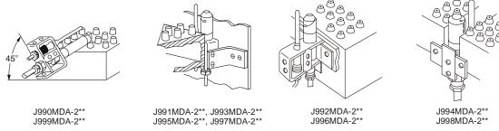
\*\* Mount pilot ignition port 1/4 in. (6.35 mm) above and 1/4 in. (6.35 mm) away from the center of nearest burner port.
