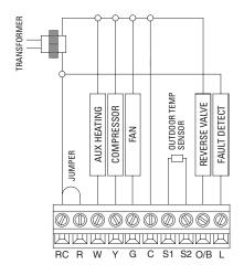
WIRING – MODEL 8465 & 8446 TWO TRANSFORMERS (REMOVE JUMPER WIRE)
