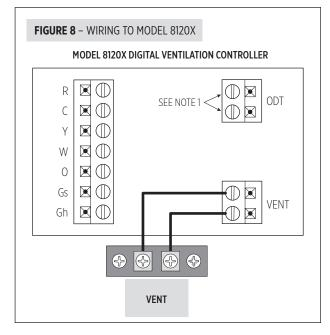
**NOTE 1:** An outdoor temperature sensor must be installed to use outdoor temperature limits for ventilation control.
