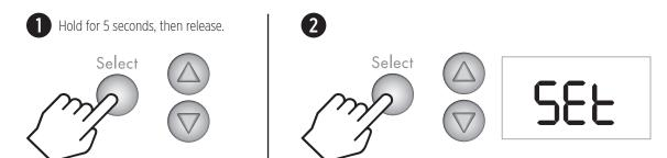
Throughout the Set Up Menu, the ▲ and ▼ buttons are used to change values, the **Select** button is used enter the value and move on to the next Set Up Menu item.
