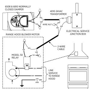
NOTE: THE MODEL 50 RELAY CANNOT BE USED WITH A DC MOTOR
