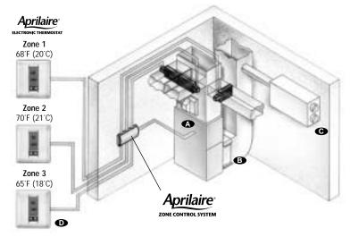
The above illustration shows a typical three zone Aprilaire Zone Control system with the following Research Products Corporation components added for the ultimate in indoor air quality and comfort:
