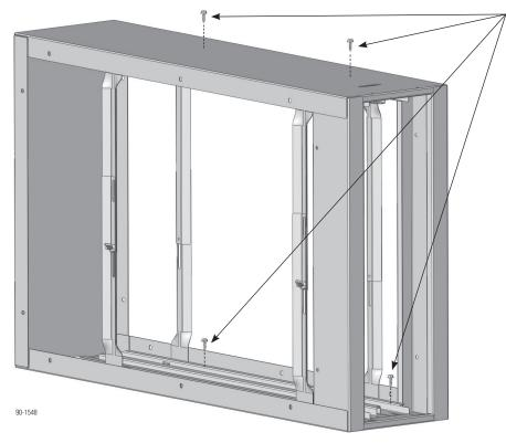
**5.** Secure the frame to the outer housing using four 1/2" long sheet metal screws.
